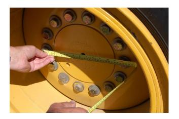
If you have an even number of bolts, such as 6-Stud, 8-Stud, 10-Stud or more: Simply measure straight across from the centre of one bolt to the centre of other bolt as shown in this photo
